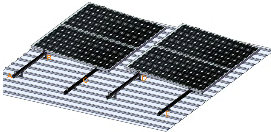
A. End Clamp B. Inter Clamp C. ECO/Elite Rail D. Rear leg E. Front leg
