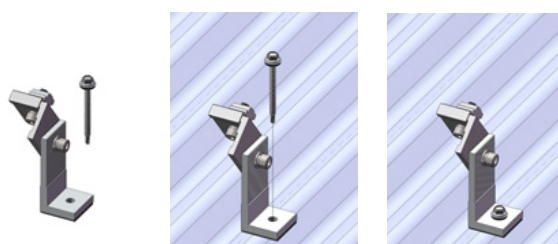
Figure 3 (Tin Foot Front Leg Installation)
