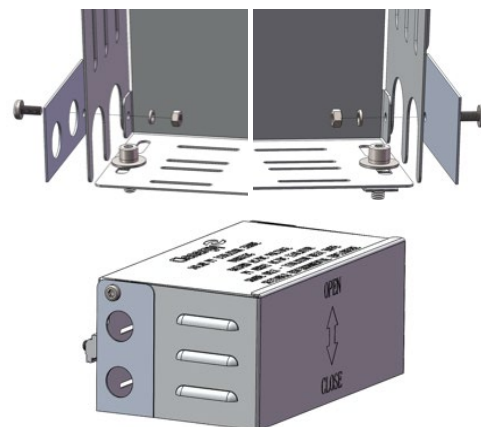
Figure 2-1 Plates Installation on Outside of Cover
