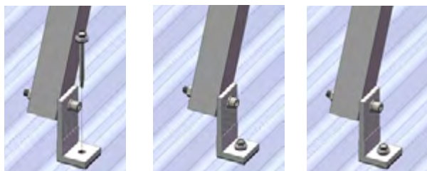
Figure 9 (Tin Foot Rear Leg Installation)
